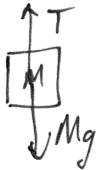
Free-Body Diagram for mass #B
