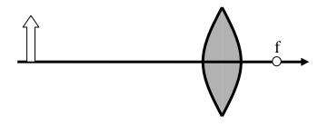
From your graph determine the location of the arrow's image by drawing a parallel ray from the tip of the arrow to the lens. At the lens continue the ray from the lens through the focal point and beyond. Next draw a ray from the tip of the arrow to the center of the lens. Continue this line through the lens. The location where the two rays intersect corresponds to the image of the arrow's tip.
