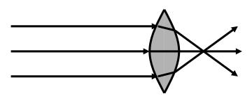
If a ray of light travels through the center of a lens, the direction of travel for the light will be unaffected. Using these two principles it is possible to determine the location of an image formed by a converging lens.
